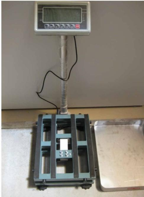
Figure 4 - Model SPB6060 Weighing Instrument
