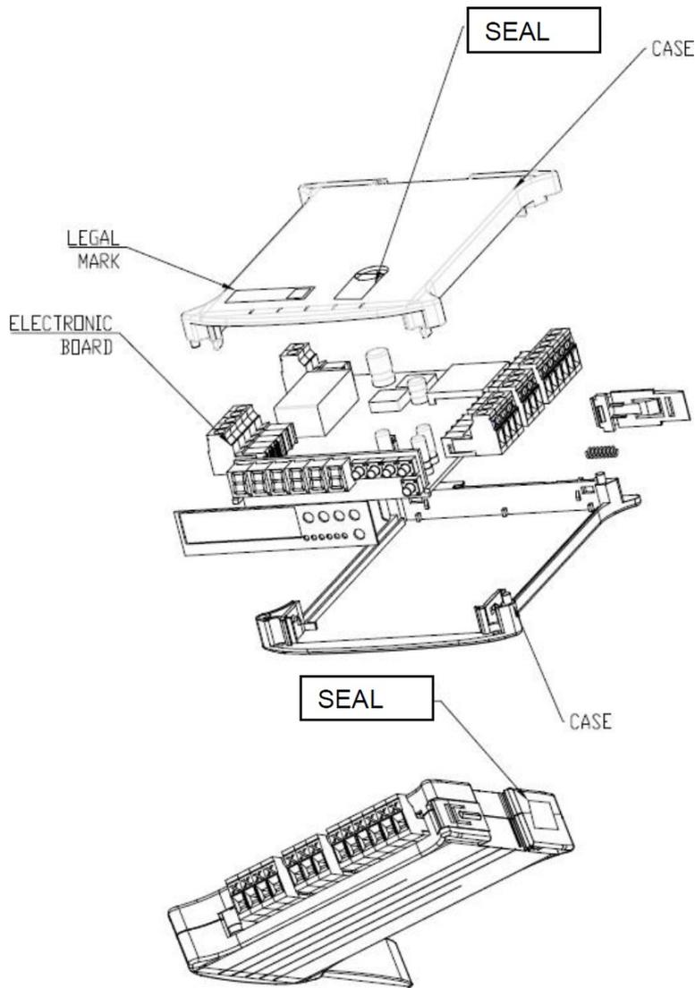
Figure 12 (Variant 1) - Model DGT100 Indicator
